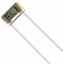
*Paper capacitors (P)* have the disadvantages of a larger variation in capacitance with temperature change and a shorter service life relative to most other types. Paper capacitors are still used for medium capacitance values of approximately 1 nF to 1  $\mu$ F, mainly at power line frequency, as for example in interference suppression capacitors.
