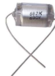
*Polypropylene film (KP)* is another excellent choice for precision and HF applications. The dissipation factor can stay below  $1 \times 10^{-3}$  to over 10 MHz. Polypropylene has a higher operating temperature (125 °C) and capacitors can be made smaller.
