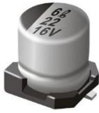
*Solid Electrolyte Aluminium* is a newer type of aluminium electrolytic, using technologies similar to solid electrolyte tantalum capacitors. Solid electrolyte capacitors have better frequency characteristics, (to > 100 kHz) and lower leakage than non-solid aluminium electrolytics. SMD implementations of solid electrolyte capacitors are increasingly being used.
