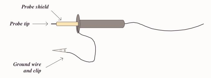
Primary factor degrading the performance of scope probeswhen used in high-speed digital electronics:Inductance of the ground wire
