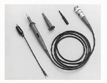
Scope probes establish a connection between the circuit under test (CUT) and the scope. Mission of scope probes: "Extract minimal energy from the CUT and transfer it to a scope with maximum fidelity".
