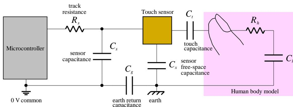
Self-capacitance touch sensors use a single sensor electrode to measure the apparent capacitance between the electrode and the 0 V common of the touch sensor circuit.
