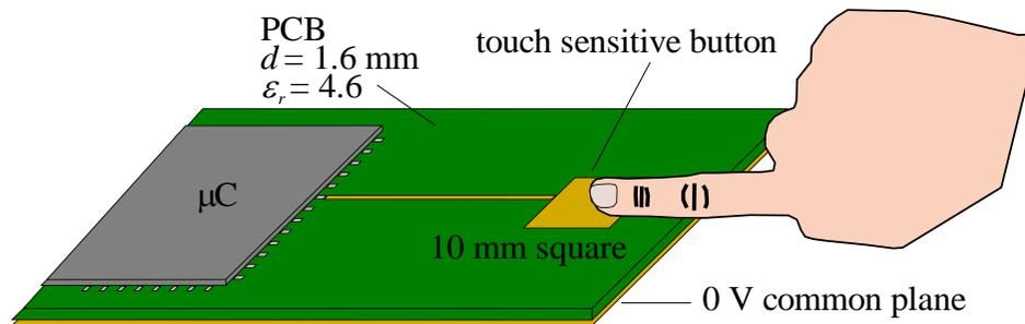
An electrical model of the system is shown below:
