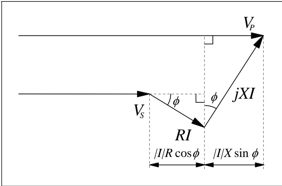
Figure 4.5 – Approximate transformer regulation
