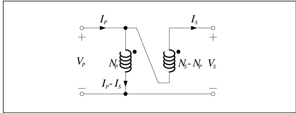
Figure 4.2 – Step-up autotransformer
