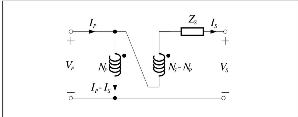
**Figure 4.3 – Step-up autotransformer with leakage impedance**
