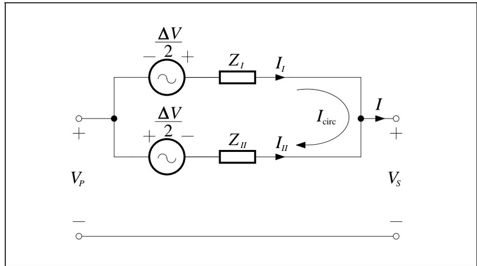
**Figure 4.1 – Two transformers in parallel**
