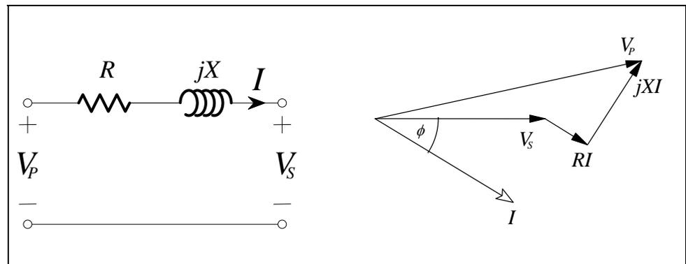
Figure 4.4 – Transformer regulation
