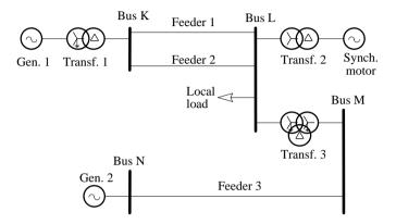
A single-phase line-to-earth fault occurs at the mid-point of Feeder 2. Assuming zero fault impedance, and neglecting all resistances, calculate the following quantities (in amperes or volts) for the duration of the fault:
