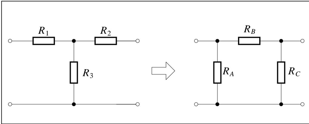
Hint:  $R_1 = \frac{R_A R_B}{R_A + R_B + R_C}$  and  $R_A = \frac{R_1 R_2 + R_1 R_3 + R_2 R_3}{R_2}$
